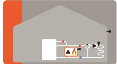
Combined storage or buffer storage with mixed heating circuit with additional function burner and boiler pump.
