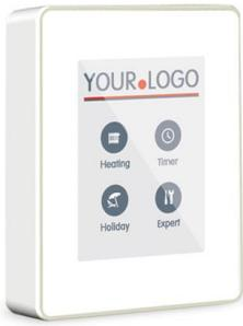
Based on our classy control panel with capacitive TFT touch display and elegant glass cover, we are pleased to develop an individual product for your application together. Using the existing hardware, operating system and various software modules is the smartest way towards your specific solution with reasonable development effort.
