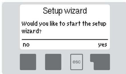
The setup wizard will rapidly guide you through the settings which need to be performed in a logically reasonable sequence. This way, any misadjustment is avoided and the parameterising is simplified.
