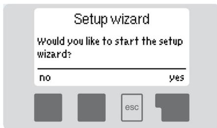
The setup wizard will rapidly guide you through the settings which need to be performed in a logically reasonable sequence. This way, any misadjustment is avoided and the parametrising is simplified.
